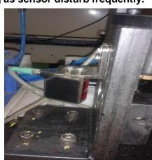
**Counter Measure: To implement banner** type sensor for showing RPM
